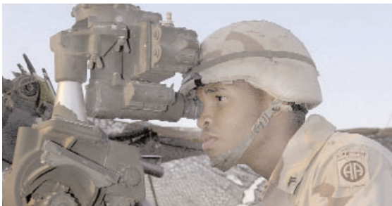
Sgt. Elijah Caddy uses a panoramic telescope to sight in a howitzer during a test fire at Baghdad International Airport in Iraq. Department of Defense photo by Air Force Master Sgt. Robert Hargeaves, Jr.
