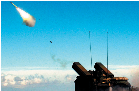
Soldiers use an Avenger weapons system to fire a heat-seeking Stinger missile during live-fire training at Pohakuloa Training Area in Hawaii. U.S. Army photo by PFC. Cheryl Ransford.
