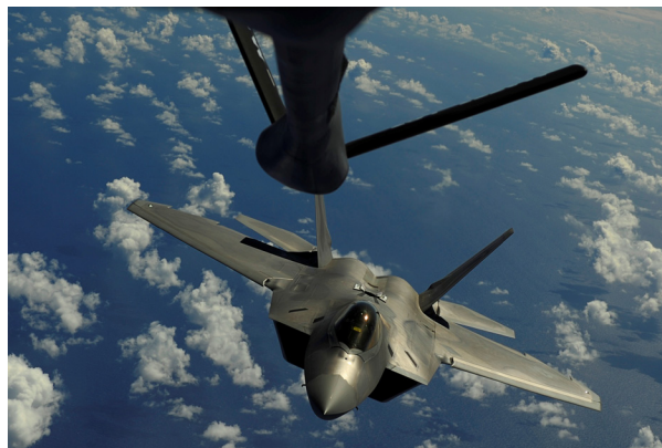
A U.S. Air Force F-22 Raptor fighter jet assigned to the 90th Fighter Squadron from Elmendorf Air Force Base, Alaska, approaches a KC-135 Stratotanker aircraft assigned to the 465th Air Refueling Squadron from Tinker Air Force Base, Okla., for aerial refueling.
