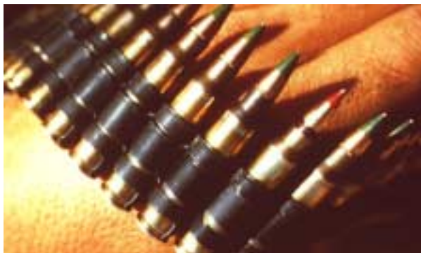
The Ordnance business manufactures and links 7.62mm ammunition for Army machine guns.
