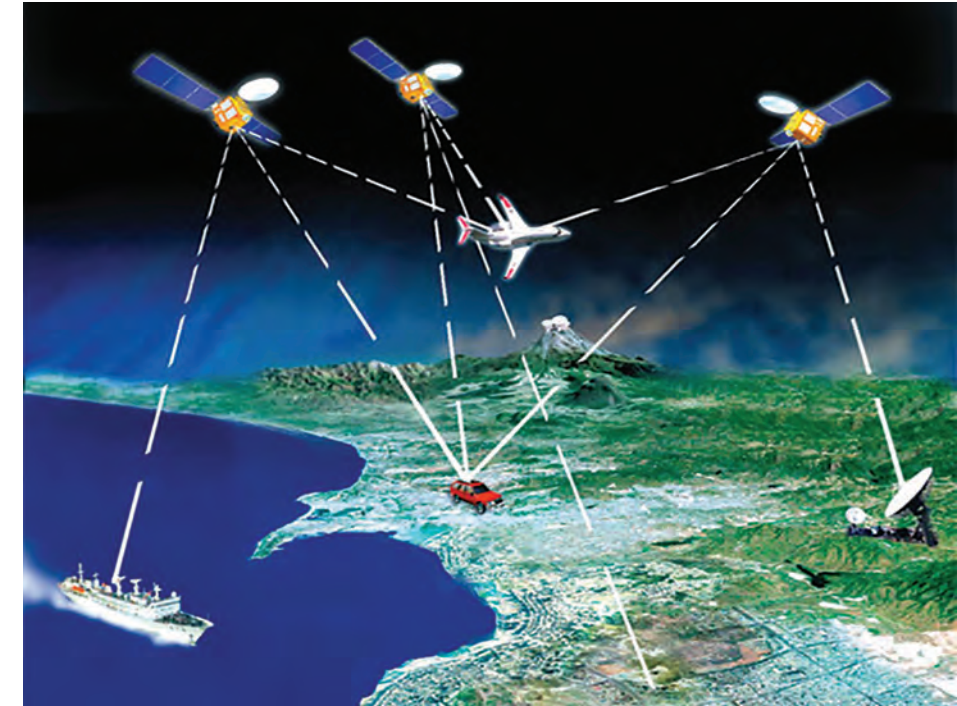
The Global Positioning System (GPS) is made up of satellites, ground stations, and receivers.
