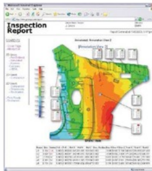
Sheet metal part reverse engineered in Geomagic Studio
