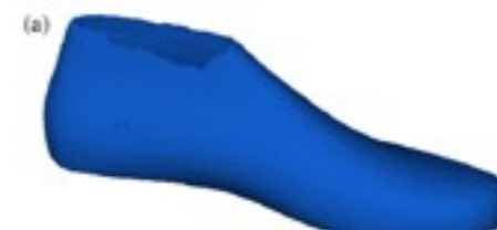
Men's Style, Length = 264.9mm, Girth = 239.3mm Basic Width = 88.3mm, Heel Height = 5.88mm
